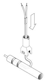
Pull excess heating cable back through standoff.
