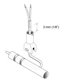
• Allow 3 mm (1/8") of heating cable to remain above top of standoff body.
