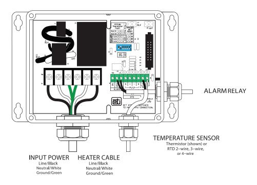
FIGURE 1. The GPT 130 wiring layout.
