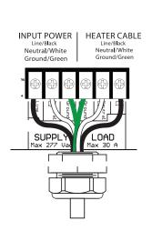
FIGURE 3. Contractor connections.
