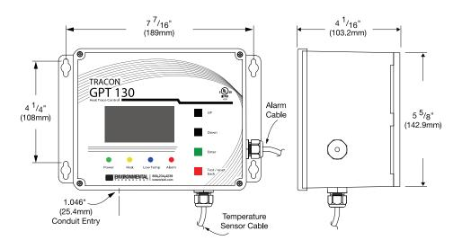
FIGURE 2. Mounting dimensions.
